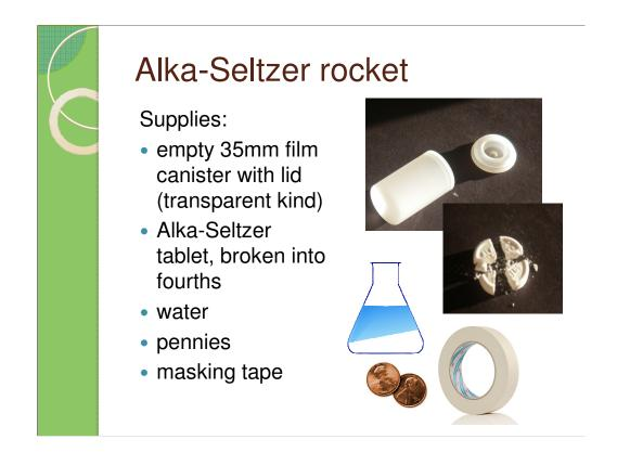
To launch a rocket, the canister is partially filled with water and the portion of the tablet is added. The lid is quickly snapped on and the rocket is inverted (lid on the bottom) and placed (normally) on a horizontal surface. After a minute or so the rocket will launch once the pressure is large enough to push the lid off. The pennies and tape can be used to modify the mass and the aerodynamics of the rocket body.
