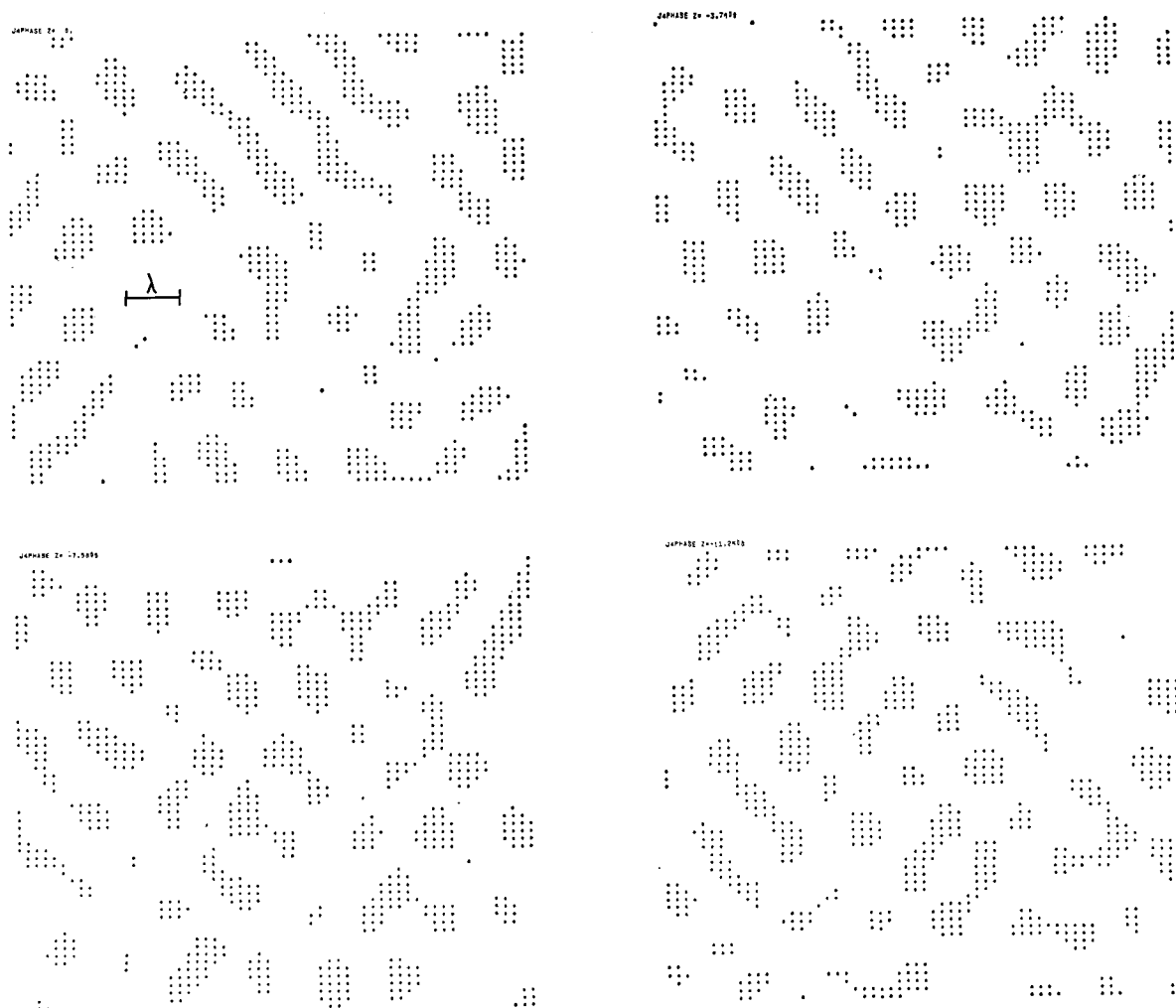
FIG. 6. A succession of computed sections through a 76:24 two-phase structure showing that connectivity of the minor phase (the asterisks) is maintained. The spacing between sections is 3.75/\beta_m . Top: Z=0 and Z=3.75/\beta_m ; bottom: Z=7.5/\beta_m and Z=11.25/\beta_m .
