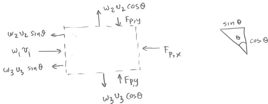
momentum balance:  $\frac{d(mv)}{dt} = \sum_i^{in} a_i w_i v_i - \sum_i^{out} a_i w_i v_i + \sum F_i$
