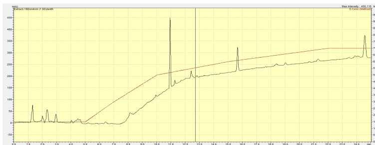
Figure A.0.2: HPLC spectrum for analysis of tar from longleaf pine litter
